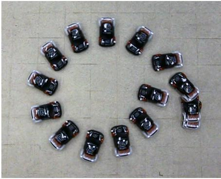
Fig. 9: Results of Algorithm 1 applied to the real drifting car. Snapshots of the car every 0.25 seconds are shown. The vehicle starts from rest and quickly enters a controlled drifting motion with a 0.8 m radius.
